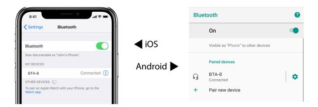
**NOTE:** You ONLY need to connect to one speaker with your Bluetooth® device (example: phone) The two speakers will automatically connect to each other & play in stereo, using their 'TWS' enabled circuit. The connect on between the two speakers MUST be made BEFORE the Bluetooth connect on to the audio source.
