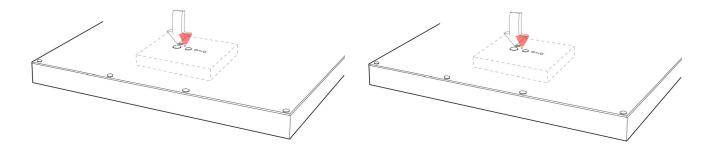
2. Press and hold the CONNECT key for approximately three seconds on one 'TWS' speaker. Its Amplifer LED Red in color) will blink. On second 'TWS' speaker, also press and hold the CONNECT key for approximately three seconds. Its amp LED will blink too.
